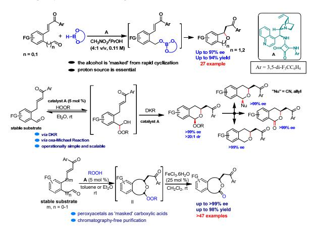
**Scheme:** a) Catalytic enantioselective synthesis of isobenzofuran and isochroman. b) Catalytic enantio- and diastereo selective synthesis of exo-peroxyacetals. c) Catalytic enantioselective synthesis of lactones.
